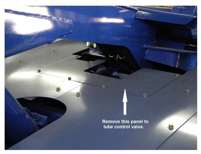
**STEP 2:** Power Wash the control valve under the boom ensuring that dirt and old grease is removed. Avoid direct high pressure power washing of values with electric solenoids
